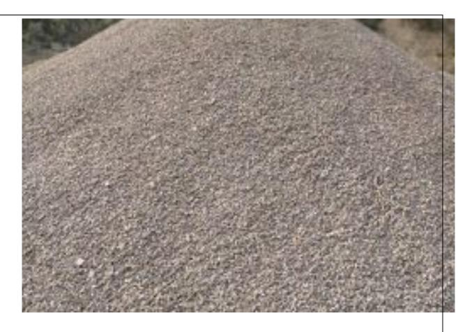
• Stone dust, this is mostly used for retaining walls and construction
